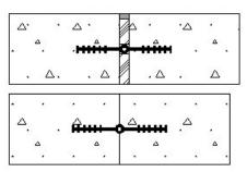
Base Seal or Rear Guard - waterstops are ideal for flat pavement jobs such as runways and large containment slab's etc.
