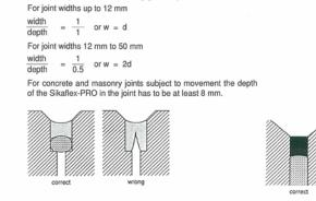
The "bottom" of the joint must not restrict the deformation of the sealant since this could result in failure during the opening of the joint. The depth of the joint should be adjusted by inserting a suitable joint backing material.
