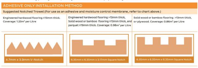
Trowel size is suggested to maximize coverage of adhesive. Periodically check coverage of adhesive during installation: >80% coverage is required for all engineered wood flooring; >95% coverage is required for all solid wood flooring or bamboo flooring products.
